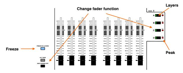
**Working with Layers** Each bank of faders has 4 layers. Therefore a bank with 8 faders can control up to 32 channels or masters. The largest surface with 44 faders can control up to 176 of these, while the smallest with 20 faders can control up to 80.
